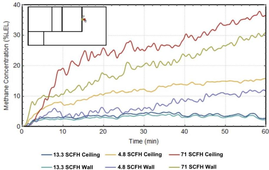
**Figure 2.** Leakage rate effects on measured concentration, 4.8, 13.3, and 71 SCFH leak rates measured at the ceiling and on the wall
