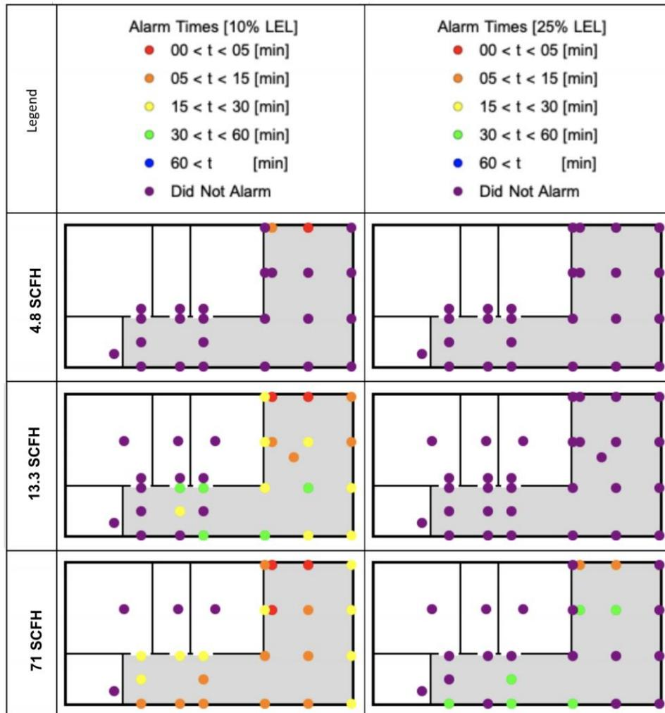
**Figure 3.** Impact of threshold concentration and leak rate on activation time for a 60 minute leak at P4 at various sensor locations
