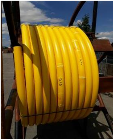
Figure 2: Coiled PE Pipe with Embedded RFID Tags
