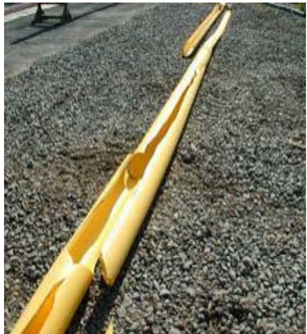
Figure 1: Crack Propagation Results in MDPE Pipe During Full Scale (Extreme) RCP Testing
