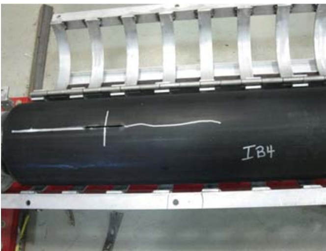
Figure 2: S4 test for RCP performed on HDPE pipe
