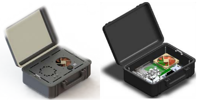
Figure 2. Model of finished mercaptans sensor with non-radioactive ionizer
