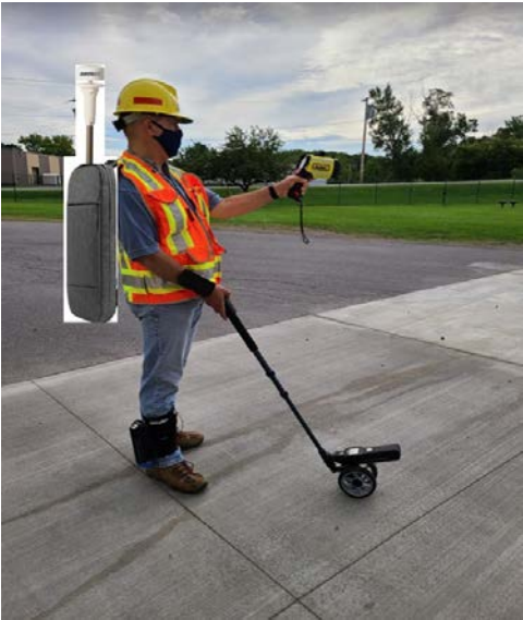
Figure 2: Simultaneous RMLD, FI/GMI and OPLS walking and wearable technologies with leak tracking identification superimposed GPS breadcrumbs on street and gas pipe maps
