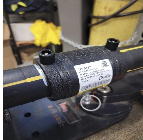
Figure 1: 2 Inch PE Pipe EF Joint
