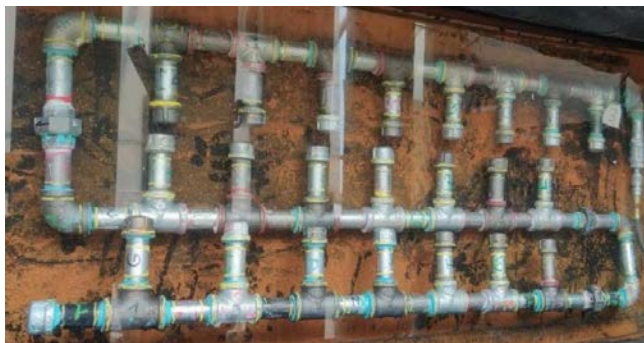
Figure 2: Sample threaded connection test configuration with different types of joints
