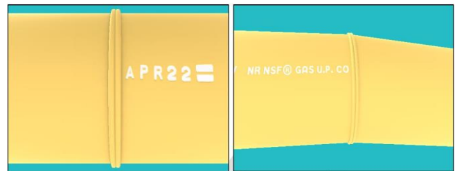
Figure 3: A Visual Field Guide example of an Illustration of an Acceptable and Unacceptable mitered butt fusion alignment
