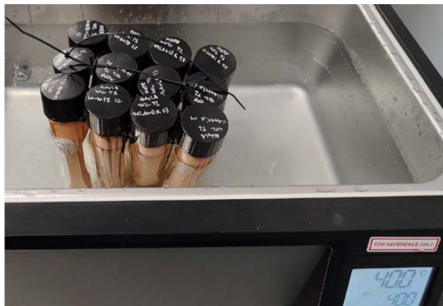
Figure 3. Water bath with extracted pipe samples submerged in testing agents
