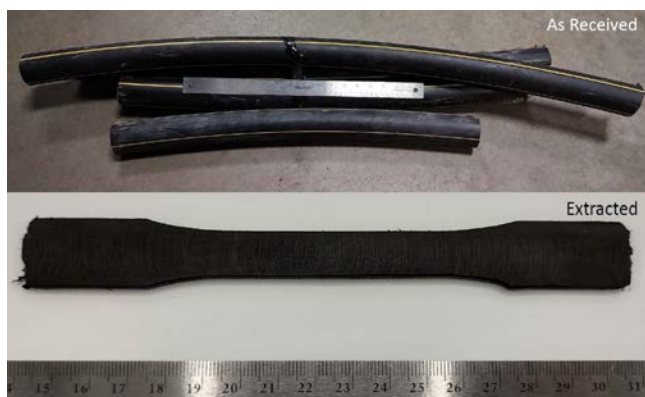
Figure 2. Extraction of HDPE pipe sample prepared for trace constituent exposure testing
