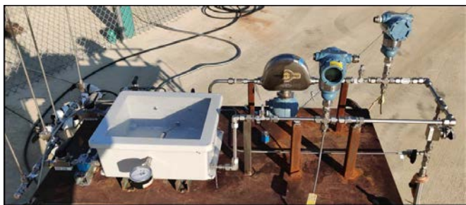
Figure 2: Example of H 2 Blended NG Flow Rig
