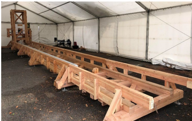
Figure 2: Test Bench with Movable Tall Tower
