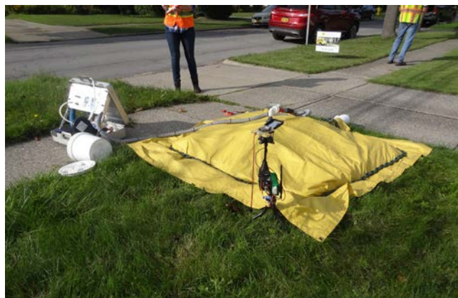
Figure 3: Closeup of one grid leak testing using SE Technique
