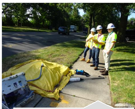
Surface area expression measurements were completed in July in National Grid territory. This project focuses on improving and standardizing the surface area expression method to quantifying methane emissions.
