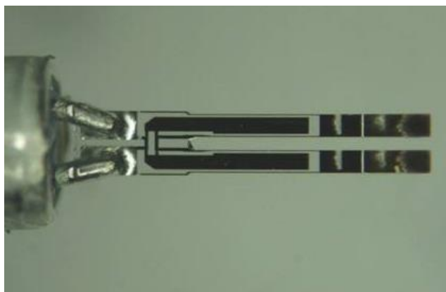
Figure 1: Tuning Fork Used in the MR Methane Sensor
