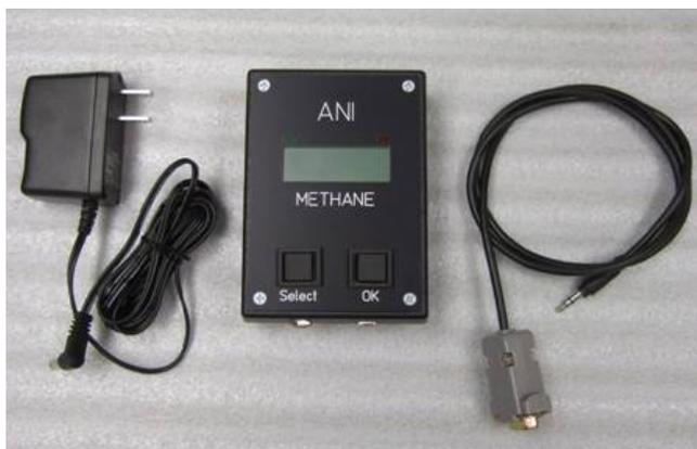
Figure 2: Engineering Prototype of MR Methane Sensor
