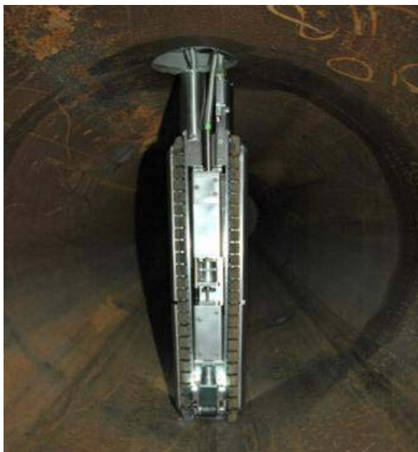
Figure 3: Entry & Retrieval via 4" Taphole
