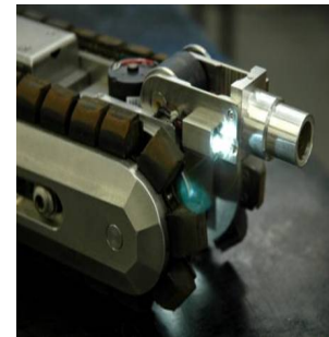
Figure 4: Pan-Tilt Camera & LED Lights
