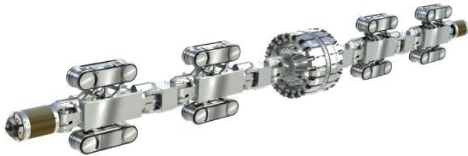
Figure 1: Explorer 20/26 equipped with an MFL sensor
