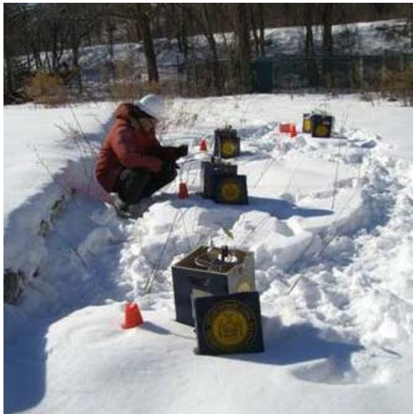
Figure 2: Soil Vapor Sampling at a Former MGP Site
