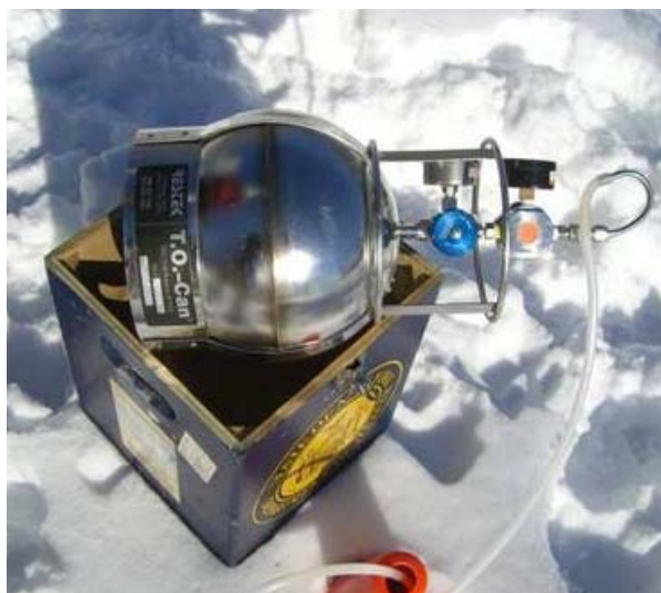
Figure 3: Standard NYSDEP Soil Vapor Sampling Canister
