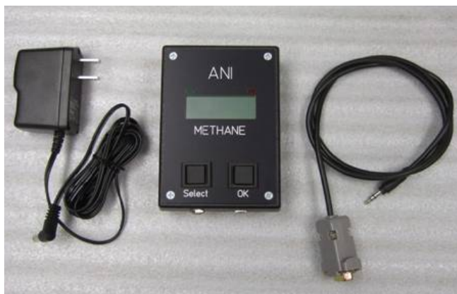
Figure 2: Engineering Prototype of MR Methane Sensor
