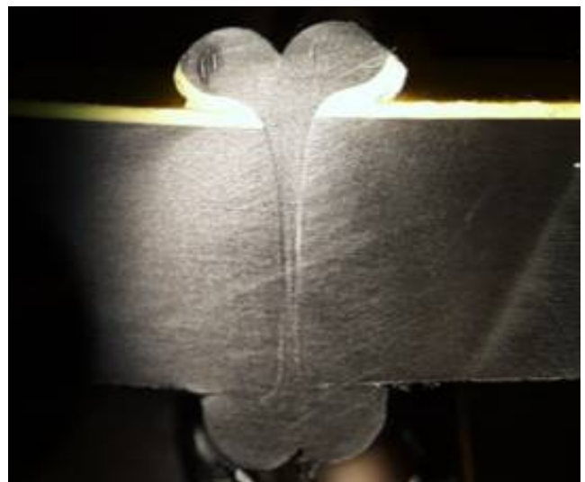
Figure 1: PE Pipe Butt Fusion Cross Section
