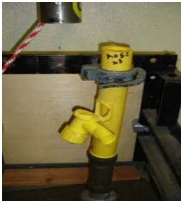
Figure 2: Impact Testing to see Effects of UV Exposure on PE Pipe Stored Outdoors
