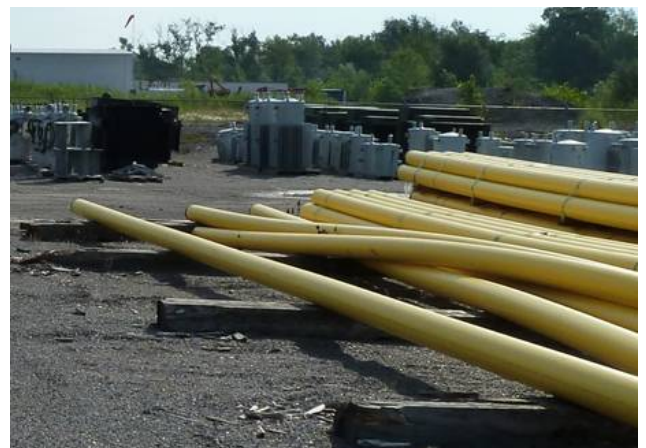
Figure 1: Direct UV Exposure on PE Pipe Stored Outdoors
