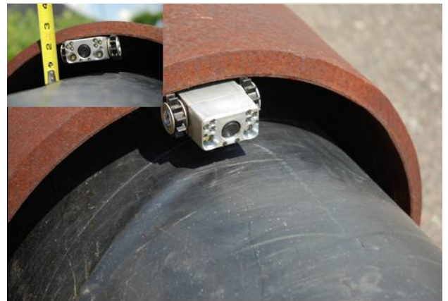
Figure 1: Shop Testing the Casing Camera Note: 1-1/2" Minimum Clearance Required
