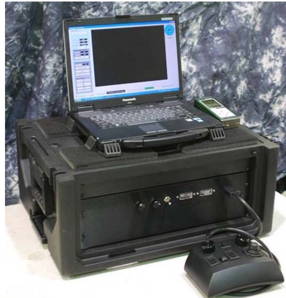
Figure 4: Control System and User Interface
