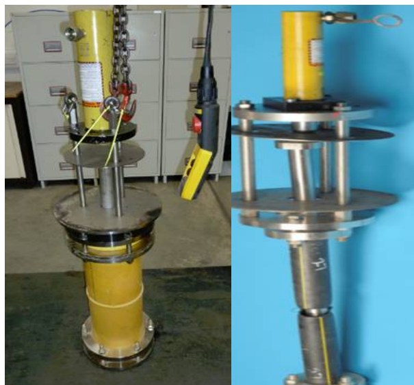
Figure 2: MDPE Specimen Prepared for WPCR Test (left), Failed HDPE Specimen Post WPCR Test (right).
