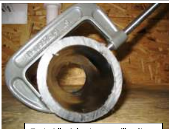
Typical Rock Impingement Test Jig Showing Internal Pipe Deformation
