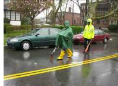
MTM Field Testing Through Asphalt & During Wet Conditions
