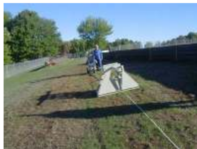
No-Pig Aboveground Inspection Test
