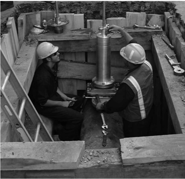
Pipeline Periscope entry tube mounted on control valve on 20-inch, 60-psi cast iron gas main during field test with PSE&G [NGA: Please note how image is cropped to maximize size of key elements]
