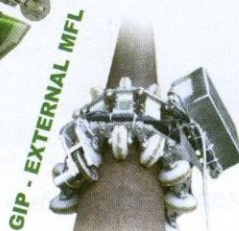
External Mount Unpiggable Lines Plant Piping
