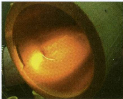
Figure 1: Slow Crack Growth.
