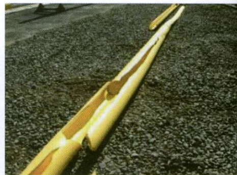
Figure 2: Results of Rapid Crack Propagation.
